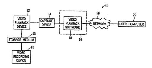
(57) Abstract: A system and method for video playback over a network includes a video playback device configured to transmit a video signal from a non-volatile storage medium and a computer coupled to the video playback device configured to receive the video signal and to transmit the video signal over a network.
