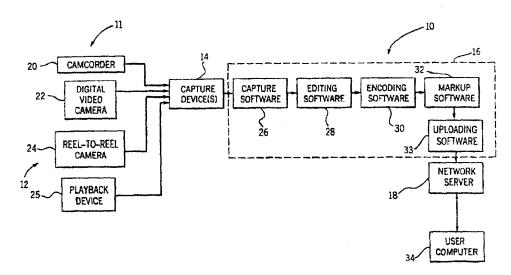
(57) Abstract: A method of streaming video includes providing a source video signal having a predetermined source video parameter; converting the source video signal to a streaming digital video file while maintaining substantially the same source video parameter; uploading the streaming digital video file to a network server; expanding the viewing frame size of the display screen to a full screen display mode; and playing the streaming digital video file in the full screen display mode.
